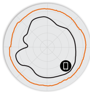
Figure 3. R730 5GHz Azimuth Antenna Patterns
