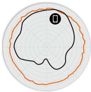
Figure 2. R730 2.4GHz Azimuth Antenna Patterns
